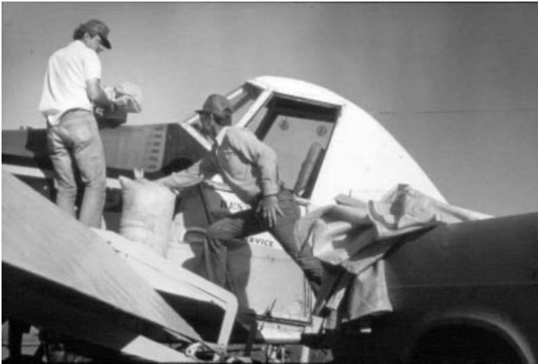
Figure VII.2-2 —The treated bran bait is sacked and then dumped into a chamber in the fuselage of the spray plane. Inside that chamber, APHIS-developed aerating equipment keeps the bran bait from clumping, which would cause uneven applications of product. (Agricultural Research Service photo by John Kucharsky.)
